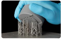
**Enhanced light touch support** structures detach from the part in seconds.
